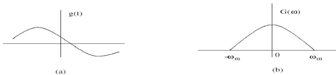
Figure 2: (a) Original signal g(t) (b) Spectrum G(\omega)
